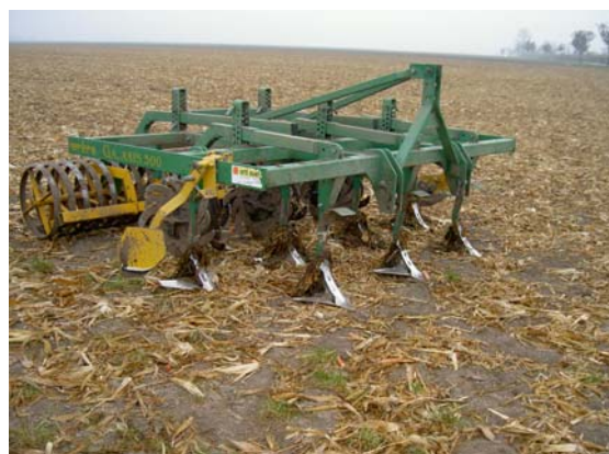
Heavy-cultivator (subsoiler) with star distributor and cracker rolls: working width: 3.0 m
