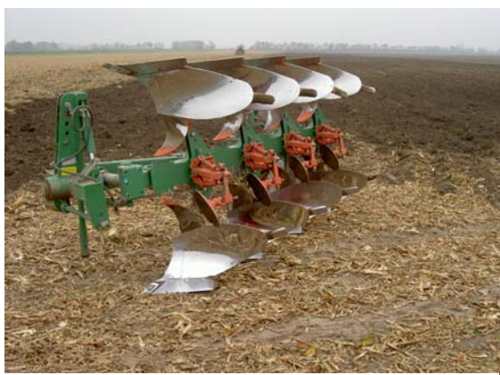
2x4 mouldboard plough – two-way-rear mounted: working width: 1.7 m
